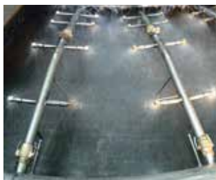
Spray bars with nozzles providing a pressure-less, balanced and efficient water cooling
