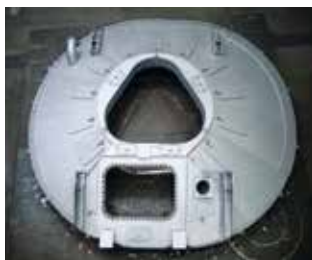
Top view of roof with holes for the electrode centre piece and the furnace elbow
